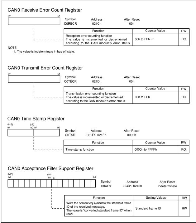
Figure 18.12 CORECR Register, COTECR Register, COTSR Register and COAFS Register
